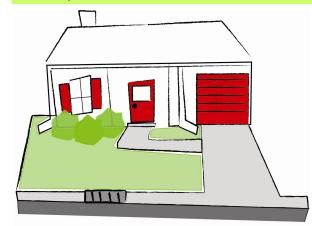
Here is a roof that pitches in 2 directions. The problem area is in the front yard, where runoff quickly exits the property and flows into a storm drain.
