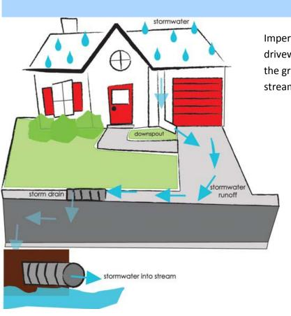
Impervious surfaces (hardscape) like roads, sidewalks, driveways and roofs prevent rain from infiltrating into the ground. Stormwater quickly enters drains and streams carrying pollutants with it.
