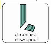
downspout and redirecting the runoff onto grass or into a garden the rainwater will infiltrate into the ground more readily, reducing runoff to the stream. It is a very simple, yet effective way to reduce stormwater runoff. Downspouts can also be directed into rain barrels or cisterns.
