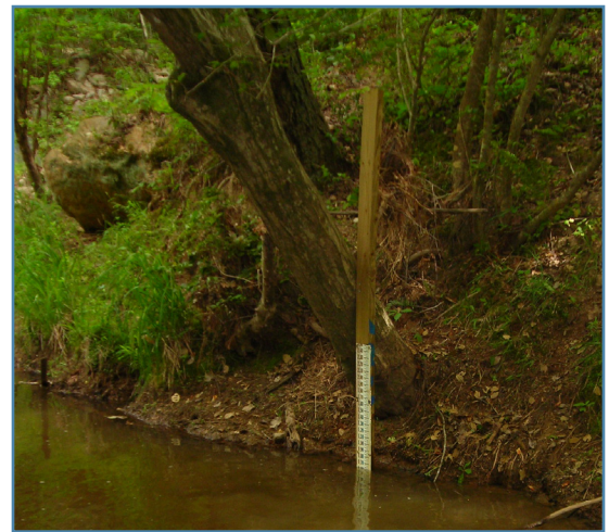
A staff gauge can be installed in the pond, similar to how it is placed at the edge of this creek, to monitor water levels and determine the wetland shelf's appropriate design elevation. (Photo: Dan Line)
