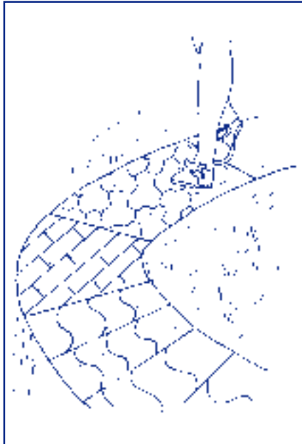
Figure 3. When installing hard surfaces, consider using porous concrete, pavers, decking, or brick pavers (shown here) on a sand base to help water soak into the soil and reduce runoff.
